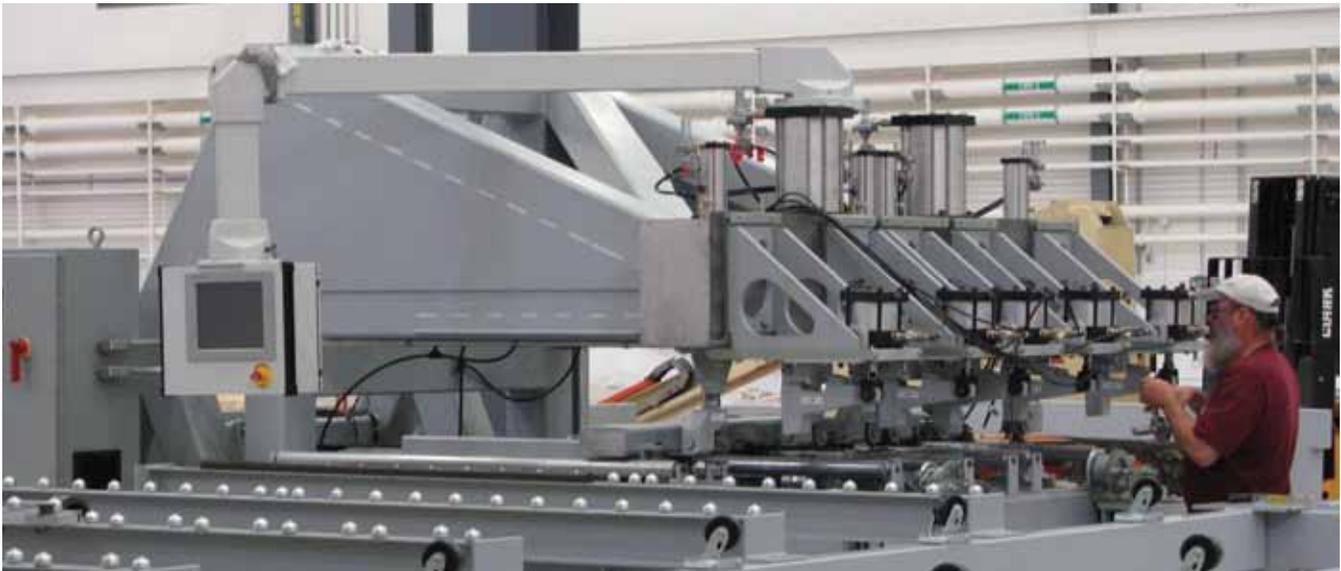
*This prototype portable friction stir welding (FSW) machine is less expensive than traditional FSW systems because its functionality is limited to the specific needs of the shipyard. This machine is shown undergoing demonstration testing at the NMC facility in Johnstown, Pennsylvania. NMC photo*
