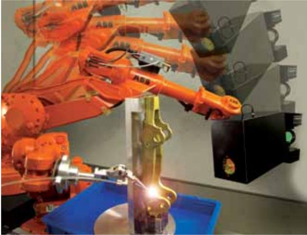
*An NMC project is optimizing the laser peening process for potential use on Navy aircraft. Shown is the robotically controlled laser beam, which facilitates uniform peening of large and complex shaped components.
