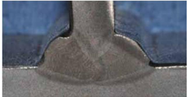
*Parameters have been determined for hybrid laser arc welding HSLA-80 T-Beams that will reduce production and assembly costs as well as improve T-Beam quality for DDG 1000. Applied Thermal Sciences photo*
