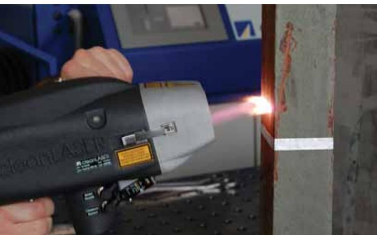
*A laser ablation paint removal system will reduce labor costs and secondary waste compared to traditional paint removal methods.
