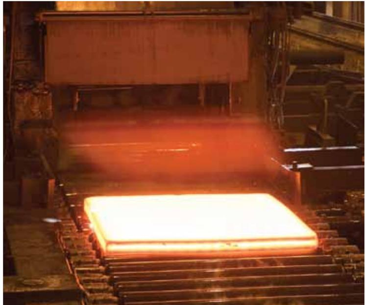
*A high-strength low-alloy steel optimized through an NMC project will be used in the construction of CVN 78, significantly reducing topside weight, which will improve the center of gravity of the ship. ArcelorMittal photo*
