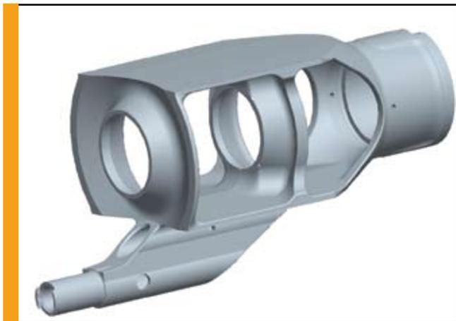
*Machined single-piece muzzle brake assembly casting. Joint Program Management Office photo.*
