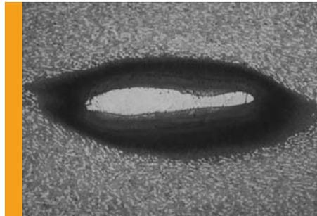
*Material defects, including hard alpha (left) and high-density (right) inclusions, can alter the effectiveness of aerospace materials. GE Aircraft Engines photo.*
