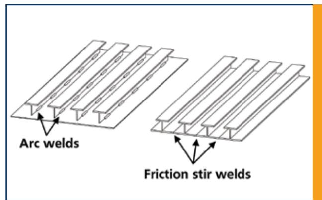
Figure 3. Sketch of arc welded construction vs. stir welded construction.
