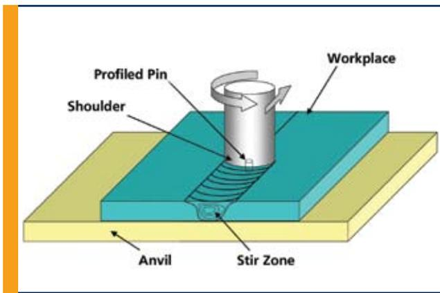
Figure 2. Schematic of the friction stir welding process.
