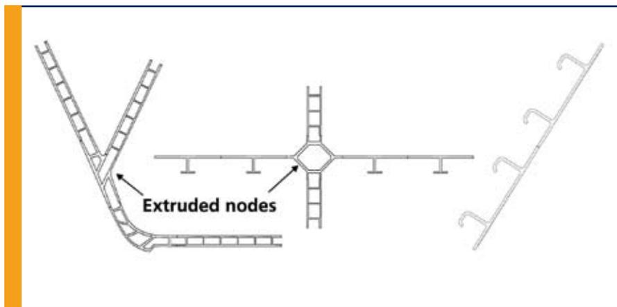
Figure 4. Examples of construction using stir welded extrusions.
