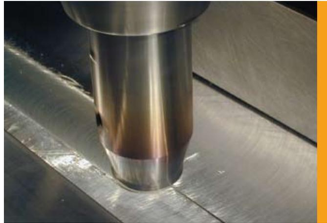
Figure 1. Welding tool plunge (left) and traverse (right).
