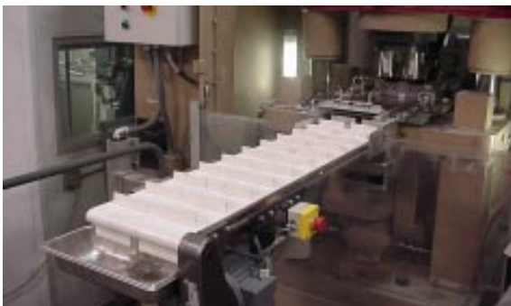
Figure 1. New cell component removal/accumulation system
