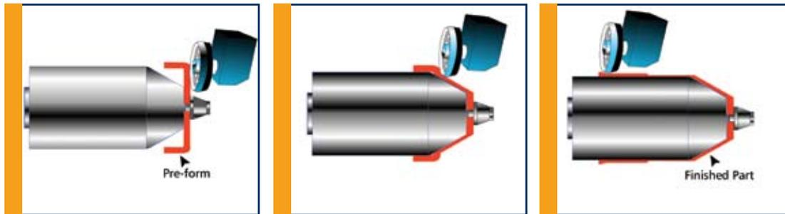
*The process (left to right) begins with a pre-form attached to a rotating mandrel. Diagram shows roller applying compressive force to the pre-form, creating the finished shape. PMF Industries photo.*
