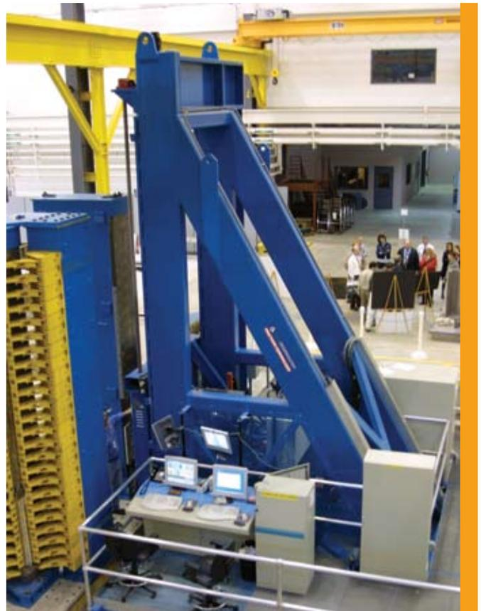
*Friction stir welding system. CTC photo.*
