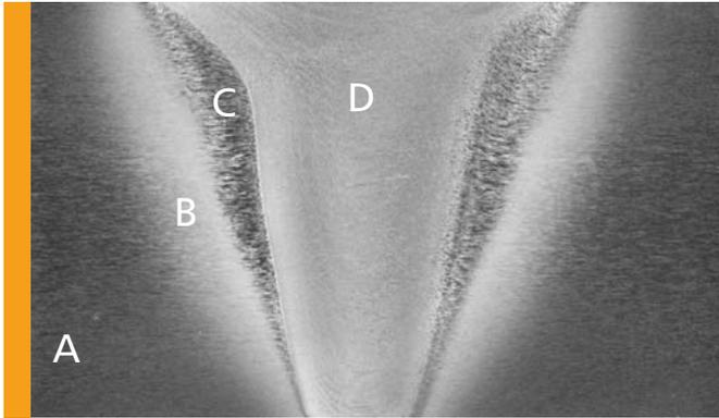
*Friction stir welding affects the welded material's microstructure, resulting in four distinct zones: the Unaffected Zone (A), the Heat Affected Zone (B), the Thermomechanically Affected Zone (C), and the Stir Zone (D). CTC photo.*
