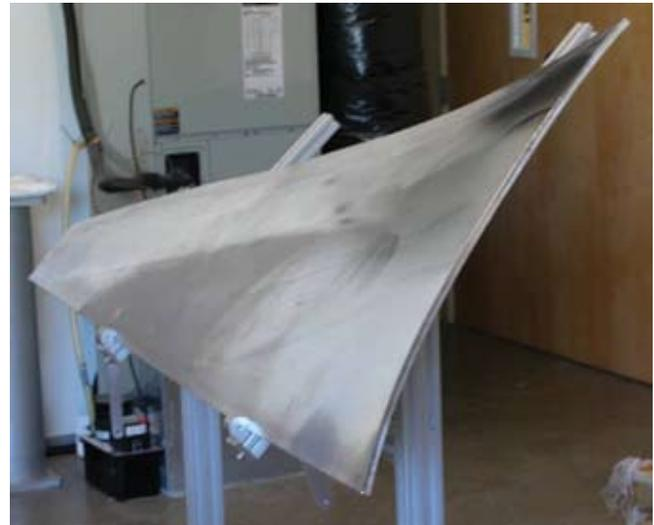
*In addition to increasing the fatigue strength of metals, laser peening is being used to form large components with complex contours for commercial aircraft. The 8 x 3-foot wing panel represented an initial demonstration of the unique processing capability. The forming process is going into production in the 2nd quarter of 2008 on wing skin panels for the new Boeing 747-8. Photo courtesy of Metal Improvement Company.*
