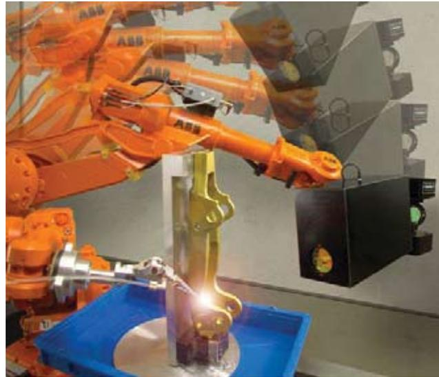
*Laser peening systems using a robotically controlled laser beam facilitate uniform peening of large and complex shaped components. Photos courtesy of Metal Improvement Company.*
