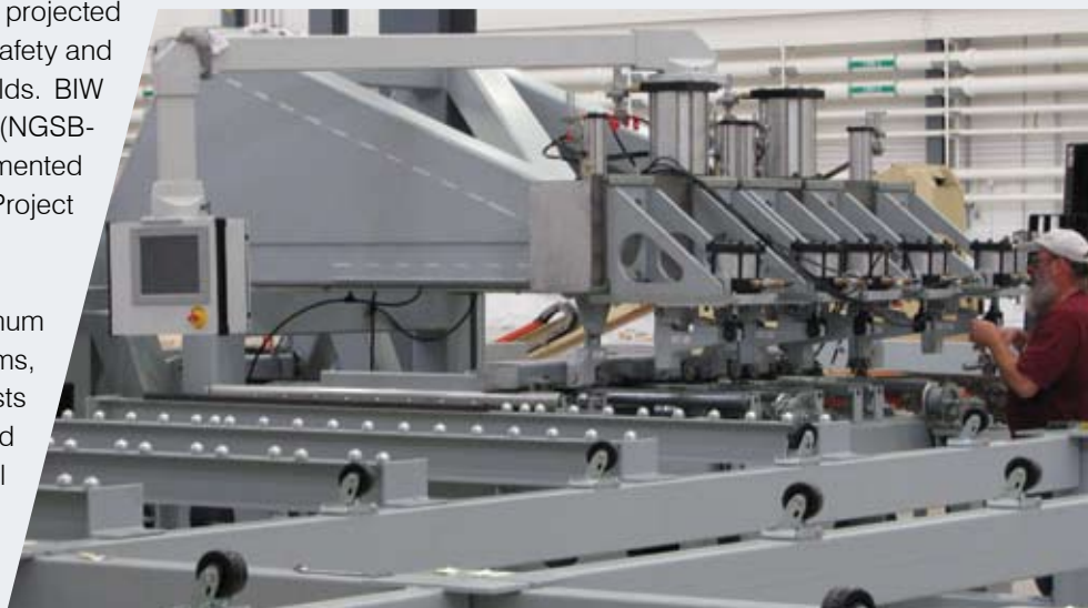
Prototype friction stir welding machine undergoing demonstration testing at NMC facility in Johnstown, Pennsylvania. NMC photo
