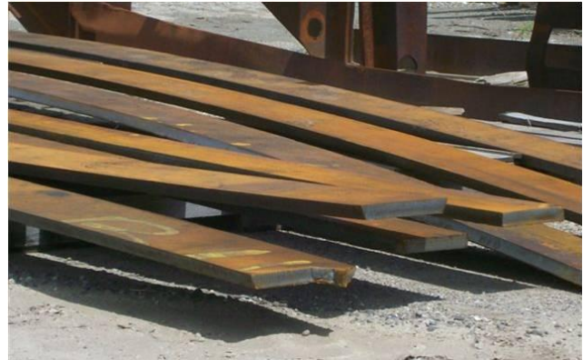
CTC reference photo. Random cut part distortion
