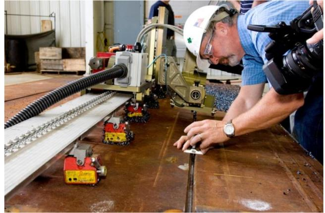
An automated back gouging tool is increasing production rates and reducing labor costs for DDG 1000 construction. BIW photo
