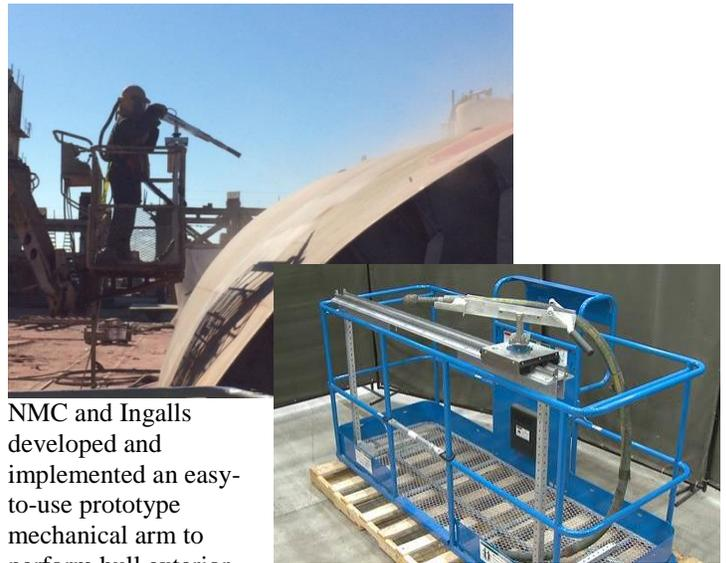
NMC and Ingalls developed and implemented an easy-to-use prototype mechanical arm to perform hull exterior abrasive blasting from a man lift during ship construction. Ingalls photo (left); NMC photo (right).
