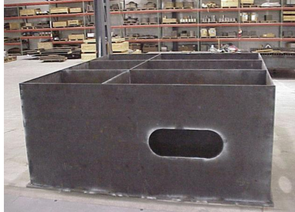
Generic ship innerbottom for comparison of distortion with computational results
