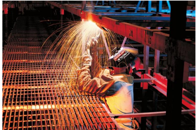
Shielded metal arc welding (SMAW) process Photo courtesy of Lincoln Electric
