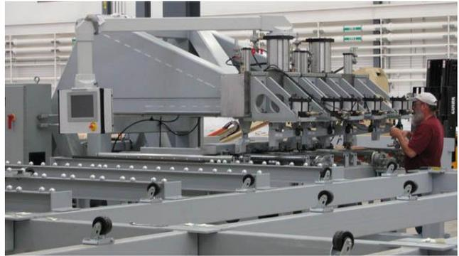
*Having completed factory acceptance testing, the prototype friction stir welding machine is at NMC for demonstration testing.*
