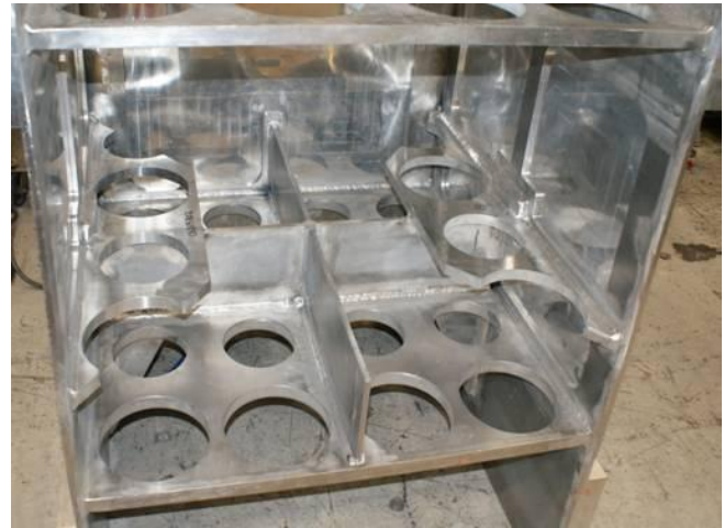
Material and manufacturing process enhancements reduce the weight and cost of the AGS pallet without compromising system performance. NMC photo
