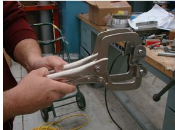
Pictured is one of the hands-free clamps that NNS is using to help reduce labor costs for manual pipe preparation and fitting processes. NMC photo
