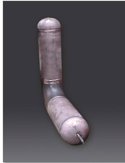
A close-die, cold forming technique was successfully applied in forming large bore, seamless INCONEL Alloy 625 pipe elbows for CVN 78. (National Technical Systems photo)
