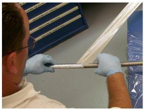
This NMC project identified and preliminarily confirmed a cryostat manufacturing process that meets Navy HTSDG requirements, which could lead to a domestic supplier. A technician is shown applying insulation to a cryostat in preparation for testing. NASA Kennedy Space Center photo
