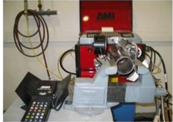
NMC developed large diameter pipe fixturing and welding process improvements that are expected to save $590K per VCS hull. Electric Boat photo
