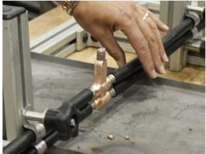
An exothermic welding process has been validated for use on CVN 78. NMC photo
