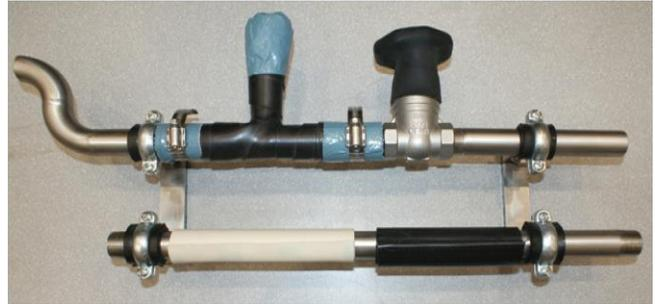
*Improvements to pipe wrapping when blasting structural steel on submarines have been identified and implemented. NMC photo*
