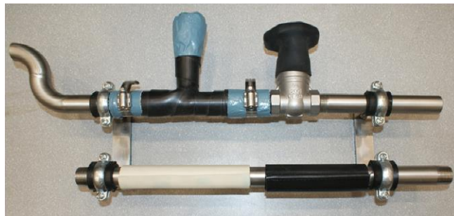
Improvements in grit blasting and the protection of piping during blasting are saving labor costs in submarine construction. NMC photo
