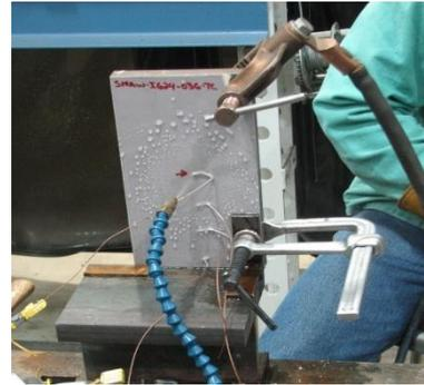
Cooling-assisted welding will prevent coating damage on the back side of plates and tank walls. NMC photo.
