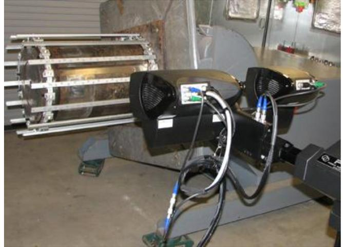
White light scanning systems can provide rapid and repeatable measurements, which will significantly reduce shipbuilding costs. NMC photo
