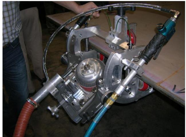
The mechanized tool will replace manual grinding of plate edges for weld preparation, which is slow and physically taxing work. NMC photo taken at BIW
