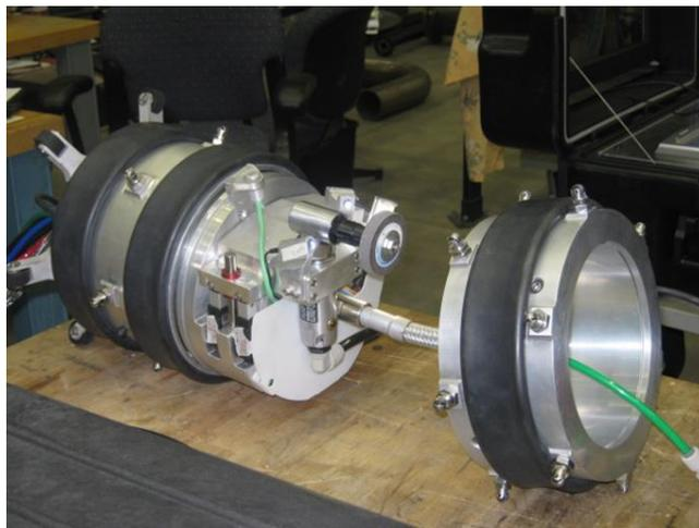
*New tools will reduce the labor hours needed to install VCS pipe assemblies on-hull. NMC photo.*
