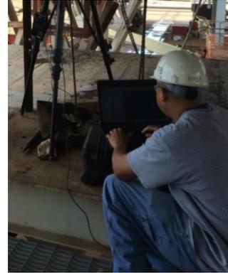
*An Ingalls accuracy control employee is pictured conducting a laser scan on a DDG 51 shaft strut to verify placement. (Ingalls photo)*
