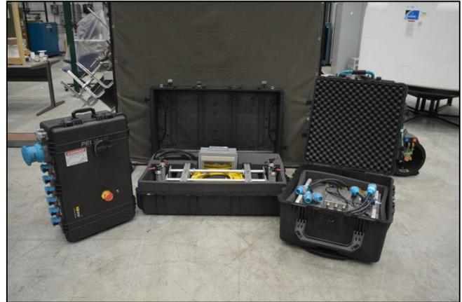
Application of a device to mitigate sensitization in aluminum structures will be less labor intensive than the current remove and replace process.
