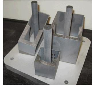
Maturing additive manufacturing (AM) technologies to produce metal electronics chassis for Navy platforms is being considered for cost, schedule, and performance benefits. (Left) internal conformal cooling channels in an AM prototype. (Right) an experimental AM build. Raytheon images.
