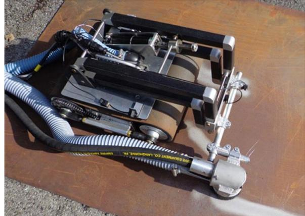
A modified remotely operated climber was developed to carry a wide variety of inspection, de-coating and preservation technologies to reduce exposure to maintenance hazards. NMC photo
