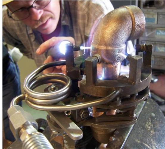
*Shipbuilding costs are being reduced by brazing pipe joints with a small, lightweight heating system as opposed to using a hand-held torch. This NNS photo shows the first CVN 78 production pipe being brazed using the new technology.*
