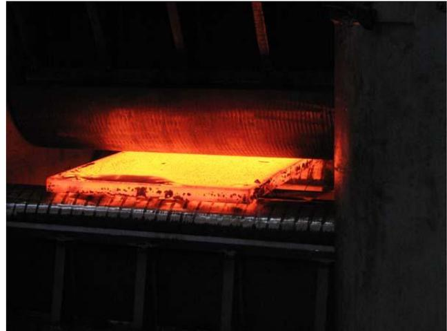
Testing determined parameters for hot forming HSLA-65 and DH-36 plates for CVN 21 and other platforms. (Concurrent Technologies Corporation photo)
