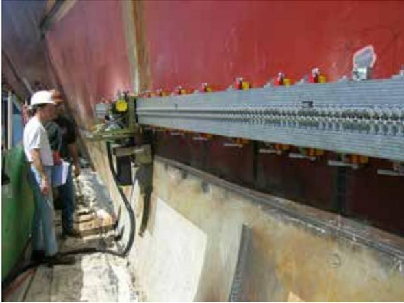
*The track weld shaver tool, pictured being tested at BIW on DDG 51, reduced manual grinding on DDG hulls. (BIW photo)*
