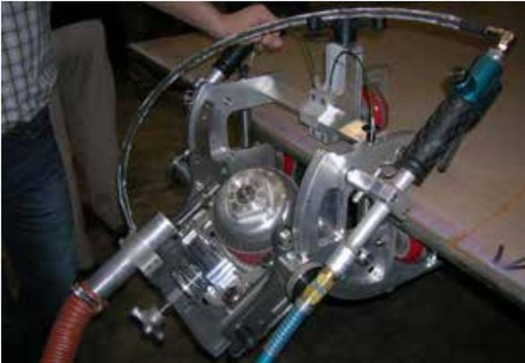
*Plate surface preparation tools are reducing the labor needed to prepare plates for welding on DDG class ships. (NMC photo)*
