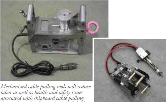
*Mechanized cable pulling tools will reduce labor as well as health and safety issues associated with shipboard cable pulling. Pictured are the capstan (top) and dual roller (bottom) tools. NMC photos*
