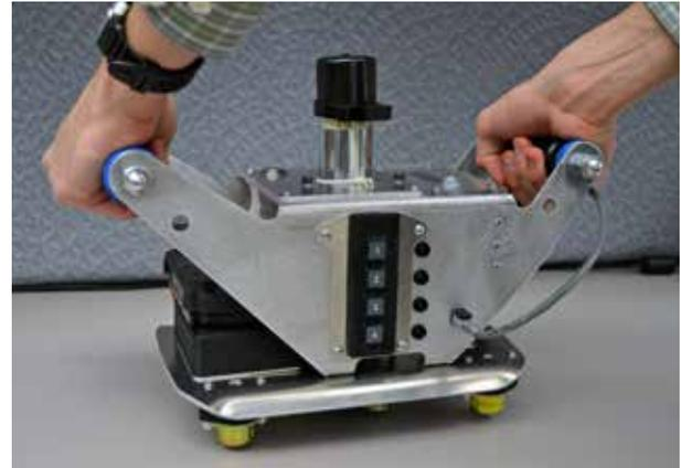
*Use of impulse hammers to identify debonded SHT areas during VCS construction is significantly less costly than correcting the problem after delivery. (NMC photo)*
