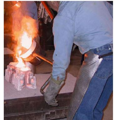
Molten metal being poured into an investment casting mold.
