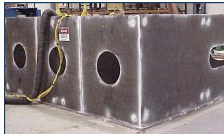
The generic ship innerbottom measures 12.5-ft. by 11.5-ft. by 5-ft. and will be used to verify two weld distortion analysis software programs.
